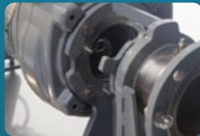
Patented telescopic inlet for easy inspection and maintenance
